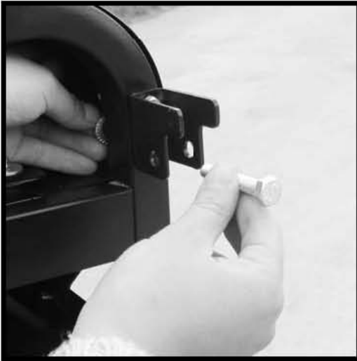
Install the handle bracket.
