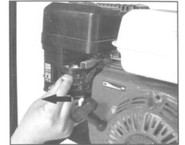
Switch the air shutter onto close position
