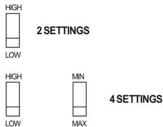
Switching from one setting to another automatically increases and decreases the wire speed and therefore the welding output. On material from 0.6mm up to 1.3mm select "Low" setting(s) and for thicker materials select "High" setting(s).
